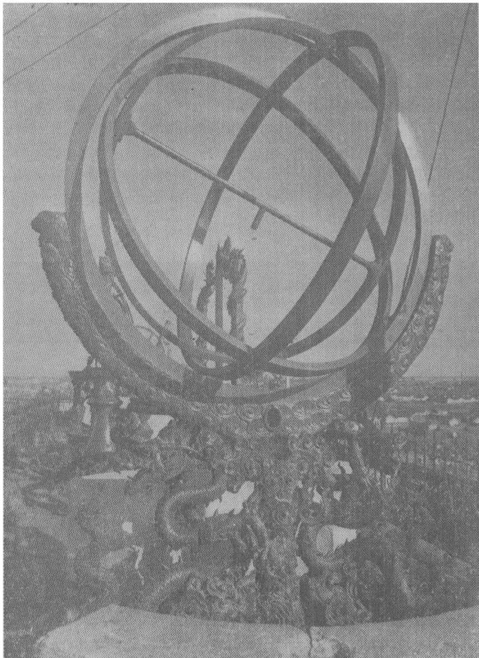
This ancient instrument, ecliptic armilla, made of bronze in 1674, was used to determine ecliptic co-ordinates of heavenly bodies
