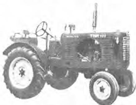
"KANCHING 25" ("Revolutionary Drive 25") 25 h.p. diesel engine Nanking, Kiangsu
