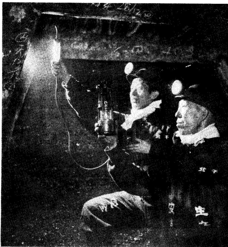
Checking for gas in the shaft.
