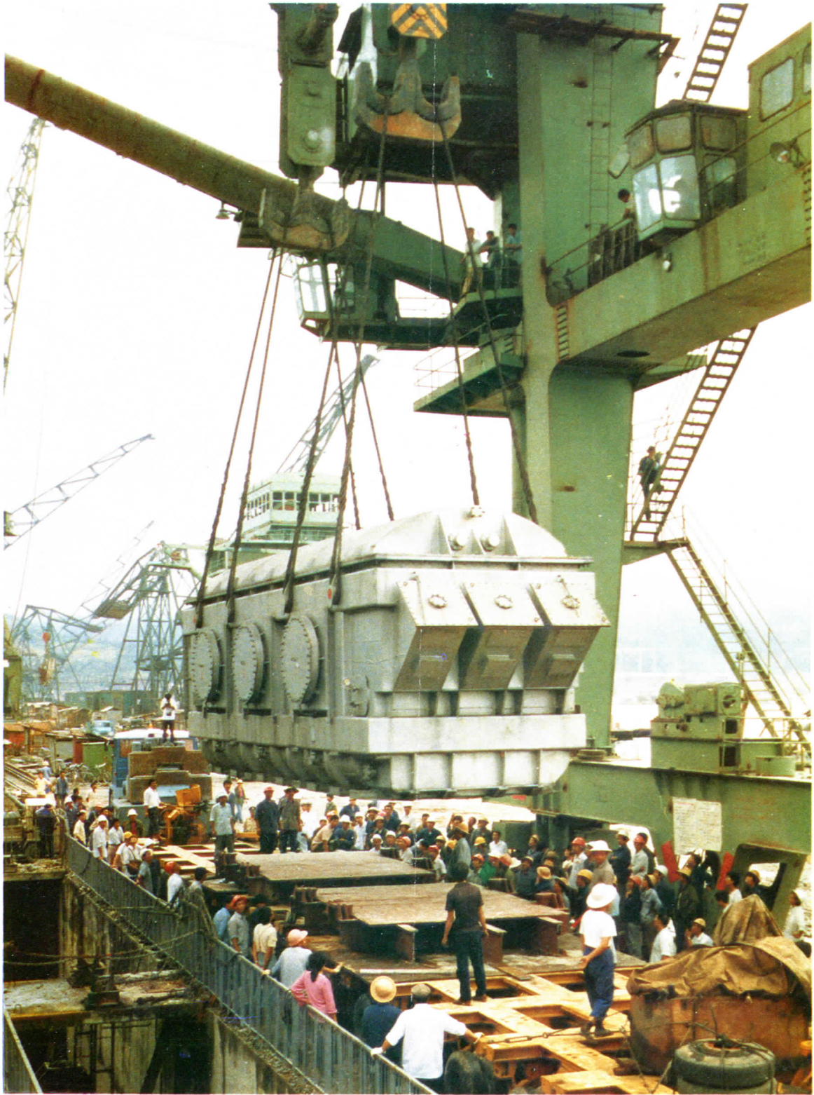
The three-phase transformer with a capacity of 360,000 kilovolt-amperes, China's largest designed and manufactured at the Shenyang Transformer Factory, was recently shipped to Gezhouba — the site of China's largest hydropower station, located on the Changjiang (Yangtze) River. This transformer, 8.8 metres long, 3.9 metres wide and 4 metres high, is one of the station's two transformers.
