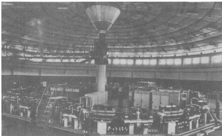
An electron storage ring in China's synchronous radiation laboratory.
